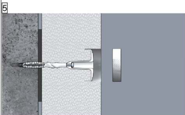
Insert the ejotherm STR - insulation cover with the help of a float
