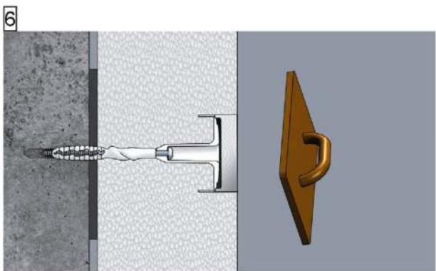
Insert the ejotherm STR - insulation cover with the help of a float
